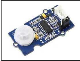
Fig. 5. PIR motion Sensor
