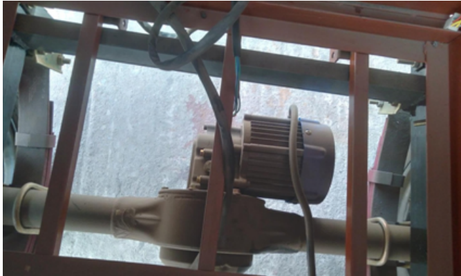
Fig. 14. Electric motor of the 6-seater Mishuk, as seen from above
