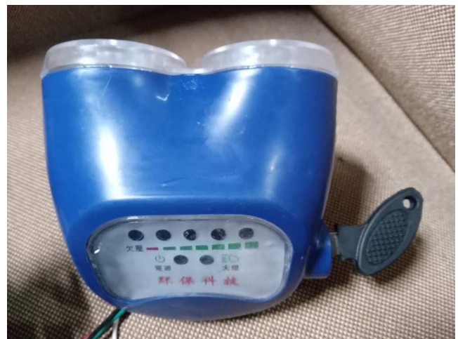
Fig. 15. The display panel, headlights and key socket are attached together.
