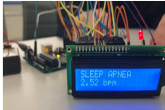
Fig. 8. LCD display of abnormal Respiration rate (apneic event)
