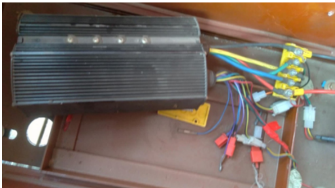
Fig. 16. The controller attached to the chassis in the Mishuk Auto Rickshaw
