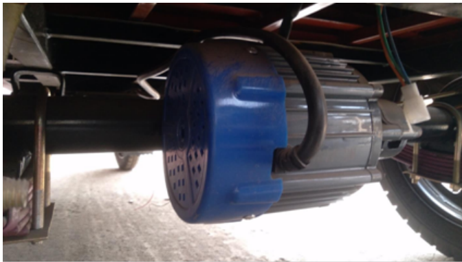
Fig. 15 . Electric motor – view from below
