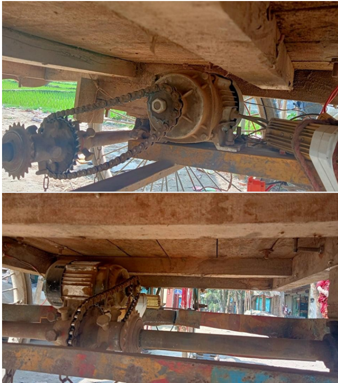
Fig. 10. Chain-driven motor for the electric van. There is no chain for riding by pedal.
