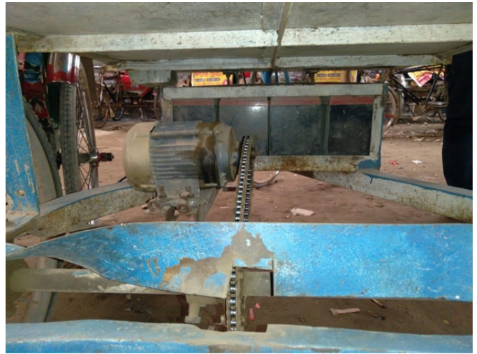
Fig. 12. Chain-driven motor of electric van, with no option to drive by pedal.
