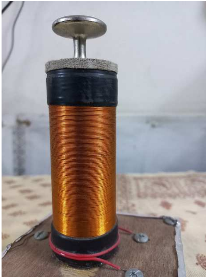
Fig. 4. The Tesla coil had 1.5 turns in the primary and 300 turns in the secondary
