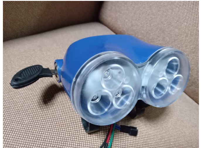
Fig. 14. the headlights with the attached key socket.
