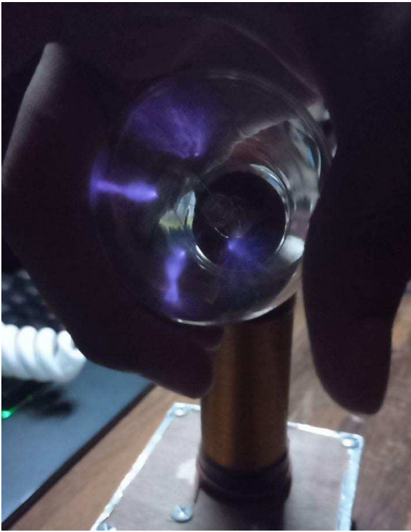
Fig. 12. Moving plasma discharge inside a common lightbulb,
