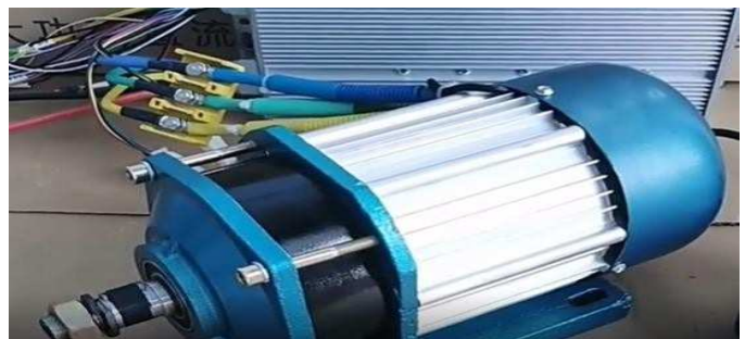
Fig 3. The larger BLDC motor used for 4-6 seater local EVs
