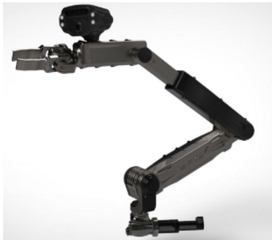
Fig. 3. 6 DoF robotic arm of the MRL team [28].
