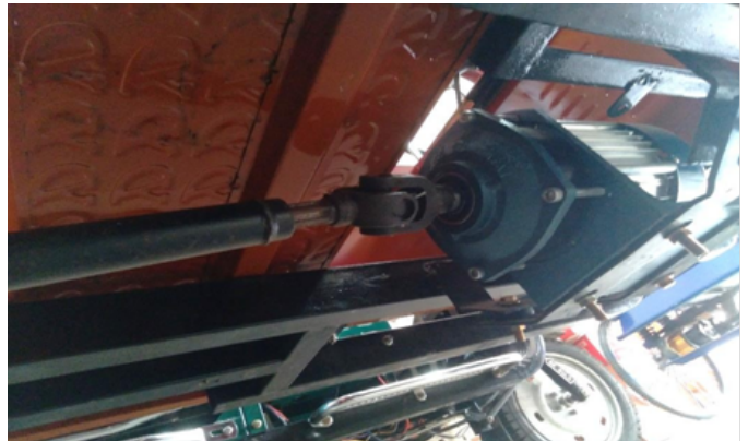
Fig. 18. The 3 kW motor and drive for the 8-seater Mishuk or Tom Tom.
