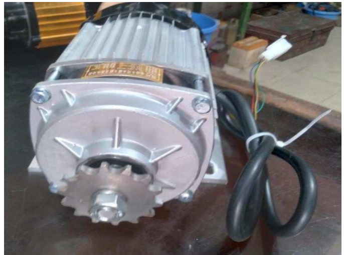
Fig. 2. The chain-driven motor setup popular in earlier electric rickshaws
