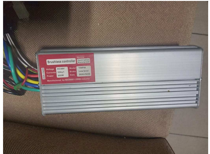
Fig. 13. The controller Yinpin , rated for 48 V, 35A \pm 1, 800 W.
