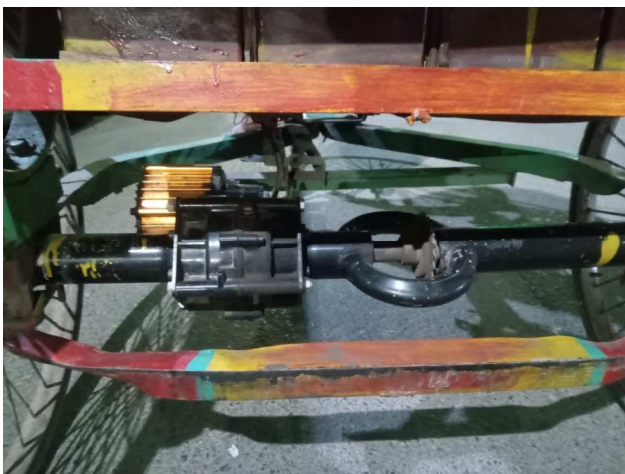
Fig. 3. A common electric rickshaw (seen in Dhaka city), with the motor (in left, gold) connected to a modified rear axle
