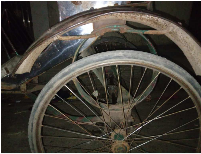
Fig. 5. The suspension is the circular iron behind the wheel and above the axle.
