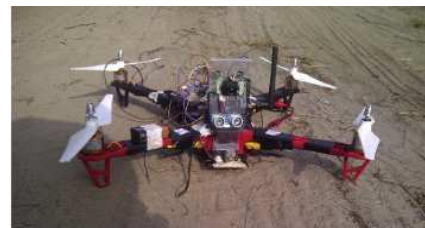
Fig. 1. E-DRONE / Quadricopter. Source: Godall Rohi, O'tega Ejofodomi, Godswill Ofualagba, Autonomous monitoring, analysis, and countering of air pollution using environmental drones, Heliyon, [2020]
