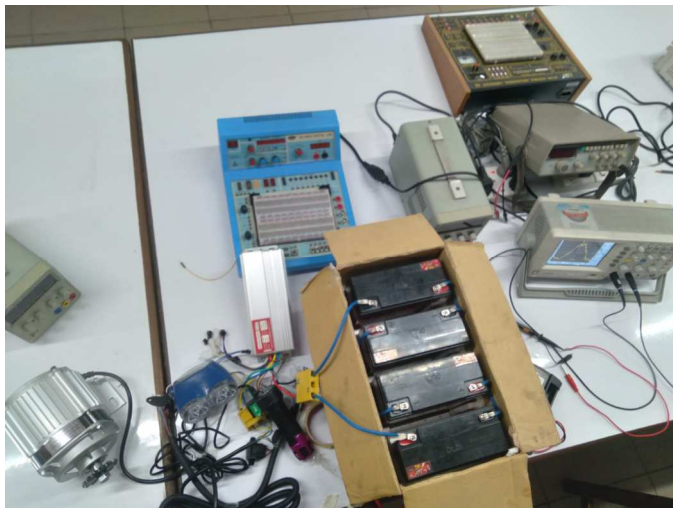
Fig 16. The batteries in series with the power electronics and the BLDC motor
