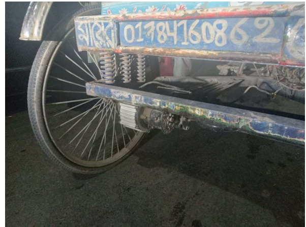
Fig. 7. Spring suspensions in a better constructed electric rickshaw. The motor and attachment with the rear axle is also visible.
