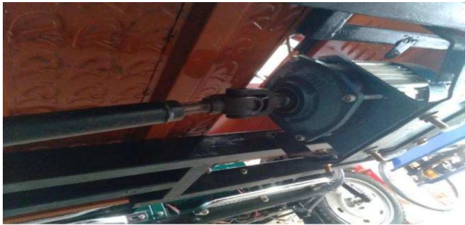
Fig. 4. The larger BLDC motor attached to the chassis of an 8-seater EV.
