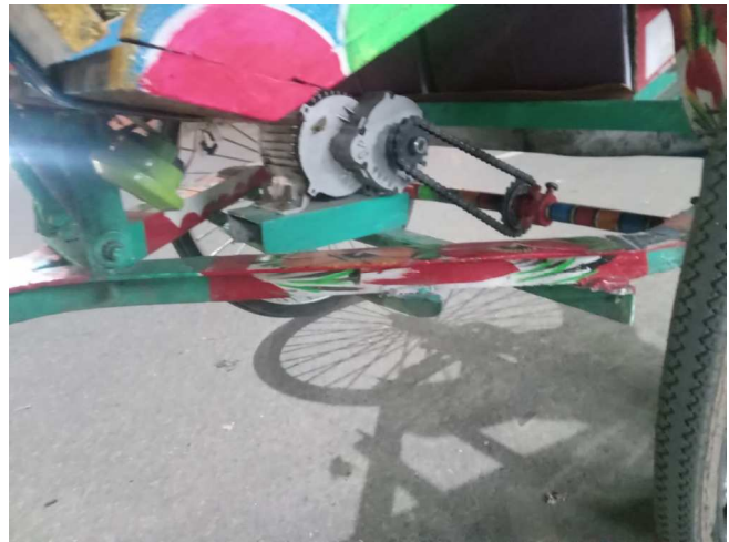
Fig 4. An older chain driven model (seen in Dhaka city) with the motor (in left, gold) connected with a chain to the axle.
