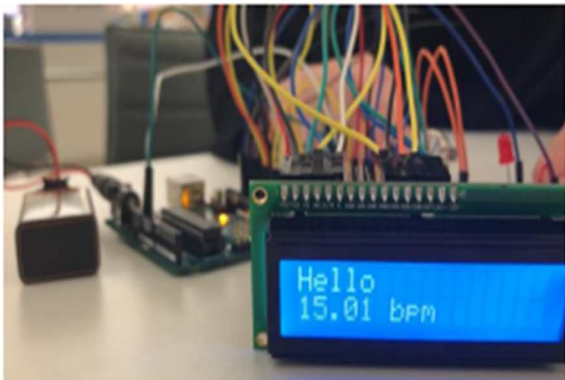
Fig. 7. LCD display of normal Respiration rate
