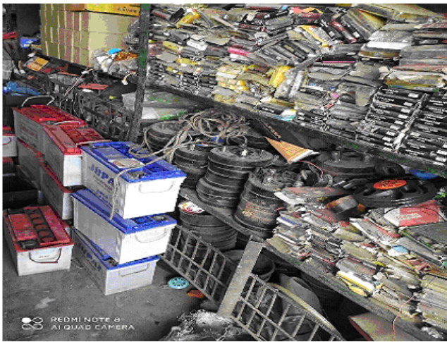
Fig. 8: The inside of a battery scrap shop, where the batteries and the lead plates are visible.
