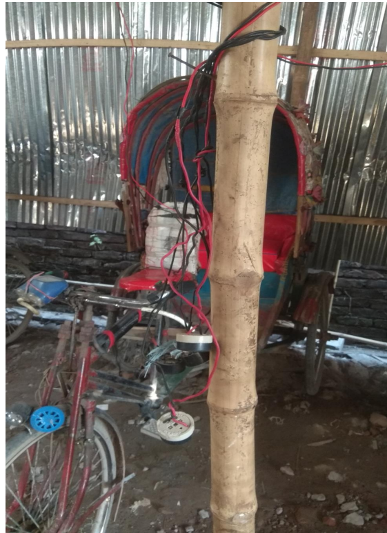
Fig. 10. An electric rickshaw being recharged
