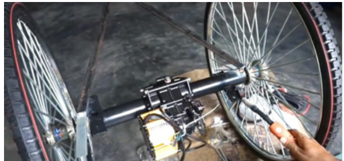
Fig. 4. The differential drive attached at the center of the axle. There is no pedal-driven chain.
