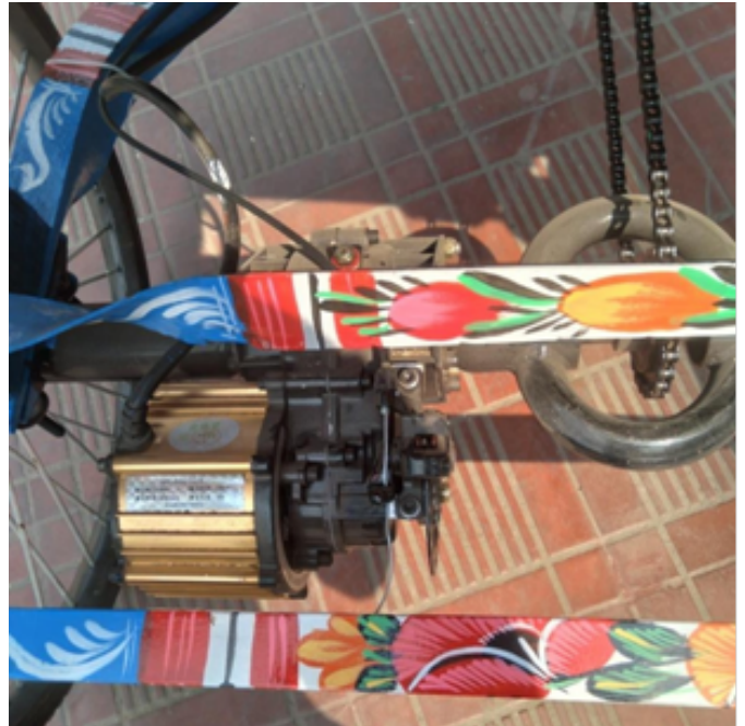
Fig. 3 The differential drive motor, with pedal-driven chain attached to the center of the rear axle.
