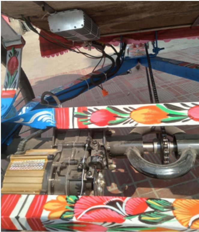
Fig. 6. Another view of the differential drive motor, with the option to pedal-drive. The silver colored controller is seen above, attached to the wooden body.
