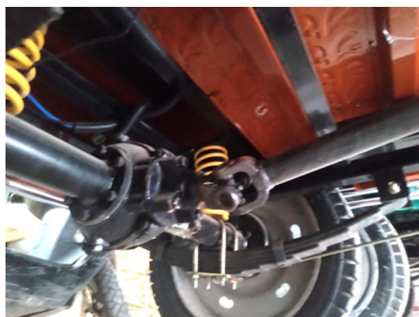
Fig. 19. The motor connected to the wheels for a Mishuk Auto/ Tom Tom. A well-functioning suspension (yellow) is also visible.
